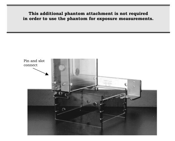
Final view of phantom assembly showing optional Lucite base support attached to phantom and placement of test tool. Note that above set-up is PA configuration.
