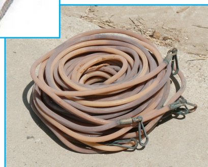
U.S. Navy Plastic Tubing (rope) with radioactive zinc sulphide
