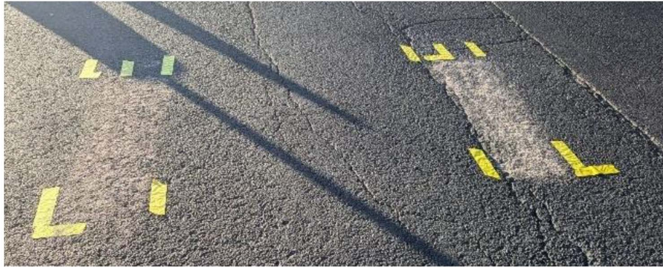
Fig. 2. Photo of the ATD seeded with a flour-sifter onto the test area prior to trials. The seeded area corresponds to the track width of the tires (1.62 m).
