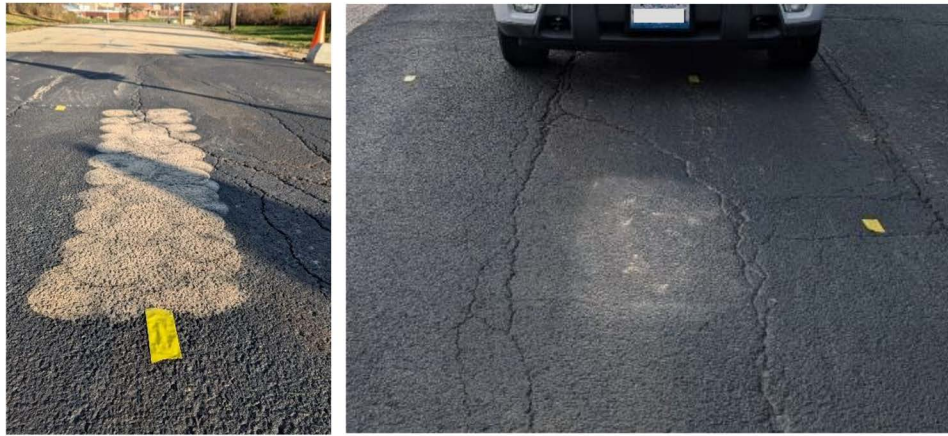
Fig. 10. Side-by-side images of the original seeding of the ground and the residual dust after four drive-over passes.
